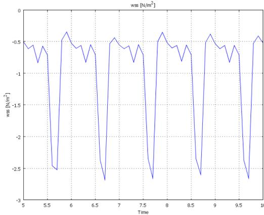
**Fig. 4** Variation (5 periods) of wall shear stress at the exit of the aneurysm with the smaller diameter (red point on figure 1)
